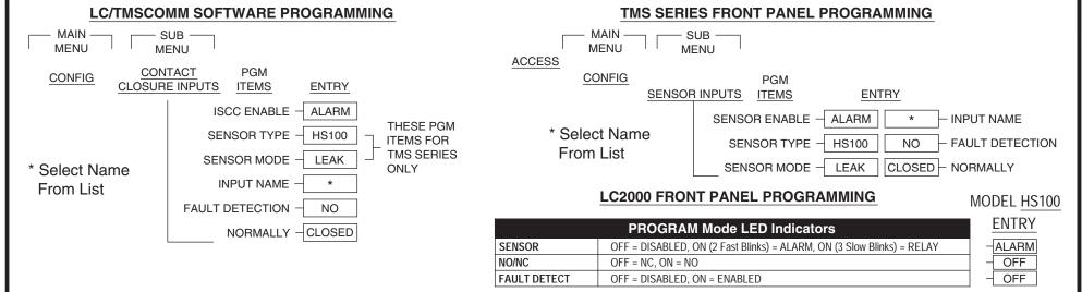
**ADDITIONAL PROGRAMMING FOR LC2000 ONLY:** Set the corresponding sensor DIP switch to "OPEN". This can be accomplished either from the front panel or via the software with assistance from PNEUMERCATOR technical support. The DIP switch is located inside the console behind the front door towards the top. Applies to both front panel and software programming
