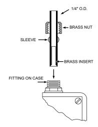
Cut off any excess tubing. Install the brass insert into end of tubing, slip first brass nut then plastic sleeve over the tubing as shown above. Insert tubing into fitting on gauge, slide plastic sleeve and brass nut down and fasten tubing securely to gauge.
