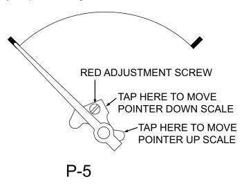
**P-5:** Remove 4 cover screws and cover. Slightly loosen the red adjusting screw. Tap the mechanism as illustrated above until the pointer indicates empty. Retighten red screw and reinstall the cover with 4 cover screws and the compression nut with tubing.
