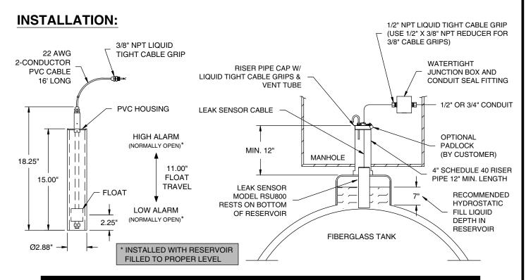
**NOTE:** Before installation, mark the sensor at 7" from the bottom. The reservoir level must be maintained at or very near this level to avoid false alarms due to level fluctuations.
